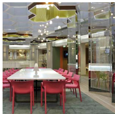
80 x 340 DOUBLE THICKNESS KINETIC GLASS PARTITIONS. © ATELIER BERNARD PICTET – PHOTOGRAPHER VÉRONIQUE MATI
